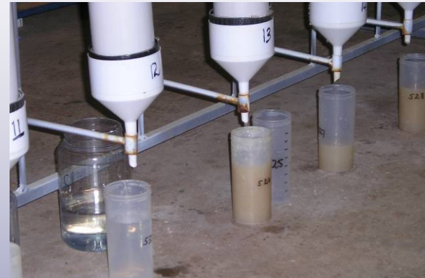
Pinhole test for compacted soils & fill. (Photo, Raine & Loch 2003).
