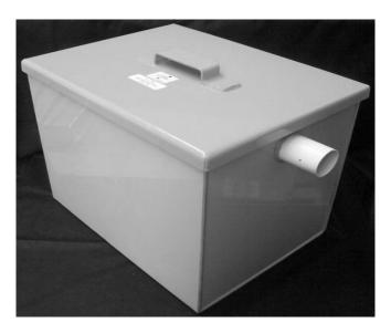
Storm Plastics Neutraliser Tank is manufactured from 6mm thick flat PVC sheet and all seams are welded using 7mm PVC trirod welding rods.
