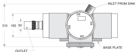
The Grease / Solids Trap - Under Sink units are suitable for small marine and inland vessels where the available area does not allow installation of a grey water storage tank, i.e. Mono Hull boats and Trailer Sailers with a small galley kitchen etc.
