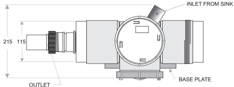
The Grease / Solids Trap - Under Sink units are suitable for small marine and inland vessels where the available area does not allow installation of a grey water storage tank, i.e. Mono Hull boats and Trailer Sailers with a small galley kitchen etc.
